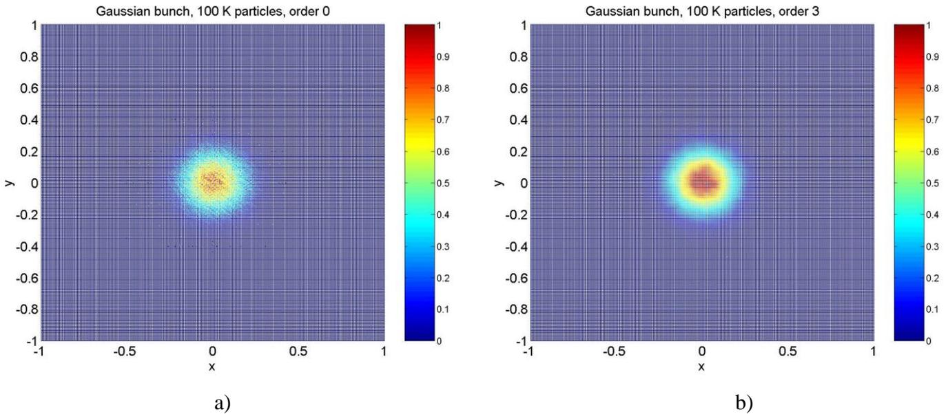
Figure 1. Space charge density calculated by the PIC algorithm for a Gaussian bunch using 100,000 macroparticles, a) order 0 b-splines, b) order 3 b-splines.
