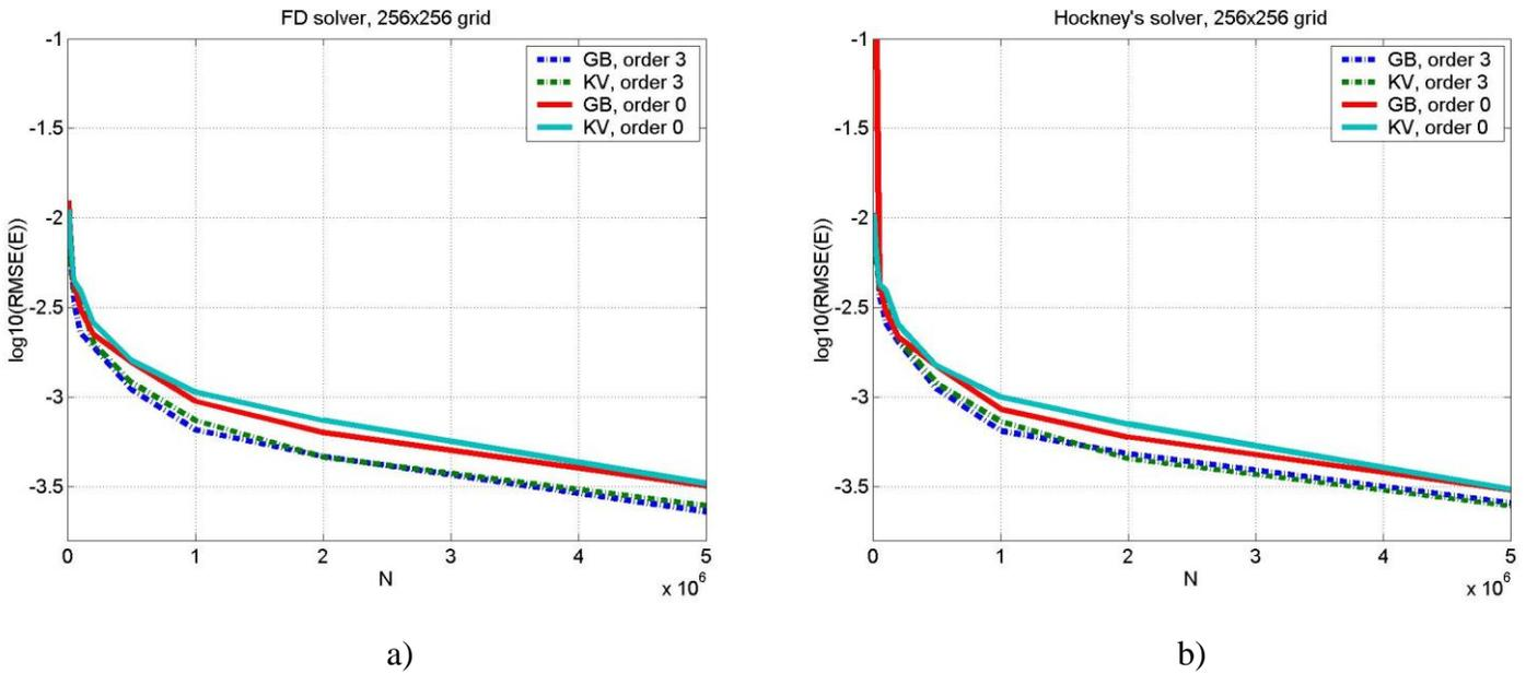
Figure 2. RMS error in electric field as a function of the number of macroparticles for the  $256 \times 256$  numerical grid, FD vs. Hockney's spectral solver, a) FD solver, b) Hockney's spectral solver.
