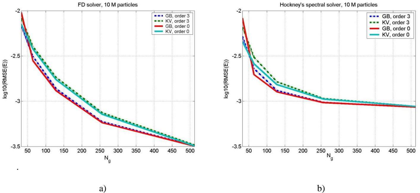
Figure 3. Convergence of the RMS of stochastic error in the calculated electric field with respect to the grid refinement, a) FD vs. b) Hockney's spectral solver, for 10 million macroparticles.
